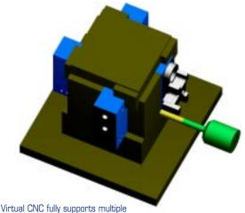
parts, fixtures, offsets, rotary tables and operations with automatic in-process stock.
