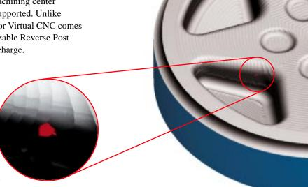
Even subtle tool collisions are automatically detected.
